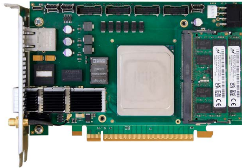
The 400GE SmartNIC designed by CESNET
