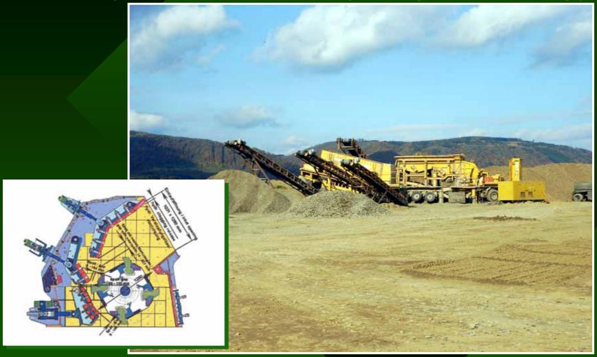
Rotation impact crusher SBM - type RCL 1232 E
