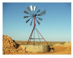
The pump could be used for pumping drinking water for livestock or water supply for farming animals, for watering the gardens with option to connect to drop
