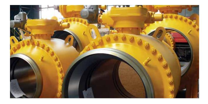
MSA, a.s., member of RIMERA Group, ranks among the world leading manufacturers of industrial valves. Production program includes ball valves, gate valves, swing check valves and globe valves according to internationally recognized standards such as ČSN, API, ANSI, DIN and GOST.
